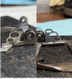
Example of the Westrock bracket mounted flush (ie against and parallel) with the existing motor mounting lip – it is hard up against the motor mounting lip, it sits in the "groove" between the motor mounting lip and the foot of the pillow block, and it benefits from some bracing from solder between the mount and the foot of the pillow block.
